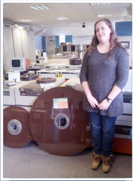
Jemima standing with some of the original hard disks – this one could store a massive 4MB per side (you'd get a single photo on this disk!).
